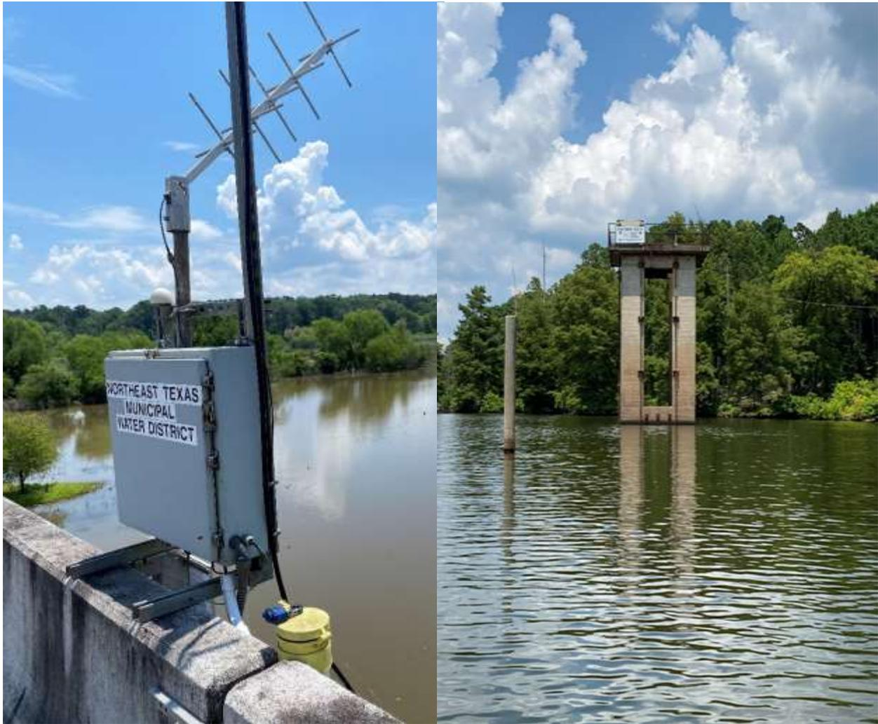
*Figure 35: US 259 (left) and NETMWD Intake (right) Continuous Water Quality Monitoring Stations*
