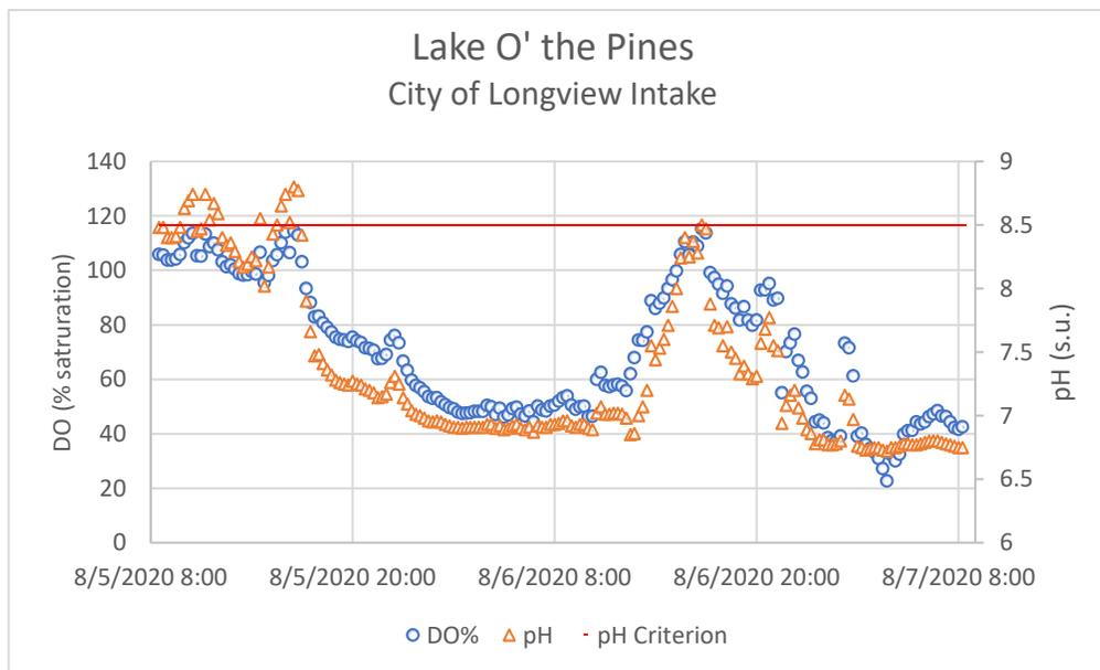
Figure 48: Lake O' the Pines: Longview Intake DO percent saturation and pH
